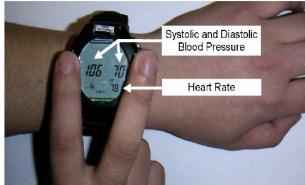
Fig. 4. Cuff-less Blood Pressure Watch Prototype (Courtesy of Poon *et. al.* [17]) Examples of 3-axis accelerometers can be found in [20, 21], and example of an integrated accelerometer/gyroscope in [6]. Kusserow et. al. presented a wireless sensor node design called
