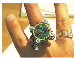
Fig. 1. Photograph of PPG Ring Biosensor Prototype (Courtesy of Asada et. al [2])
